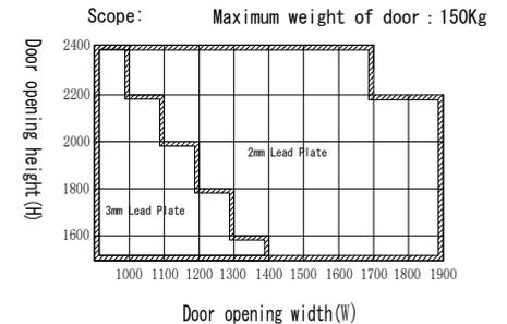
Remark: It need to adjust the height of waist plate, when opening height is over 2200mm.
