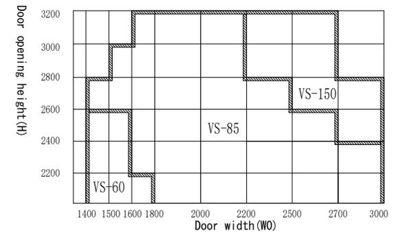
Remark: The range is only base on 10mm glass. Calculation is necessary for other glass thicknesses.
