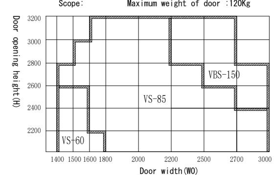
Remark: The range is only base on 10mm glass. Calculation is necessary for other glass thicknesses.
