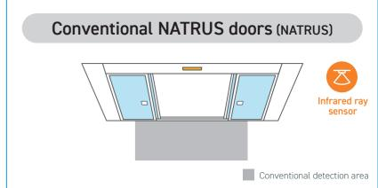
By the adoption of an image sensor: The sensor detection area has expanded 4 times
